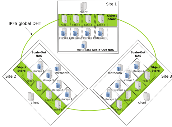
Fig. 15. Topology used to deploy an object store on top of a Scale-Out NAS local to each site.
