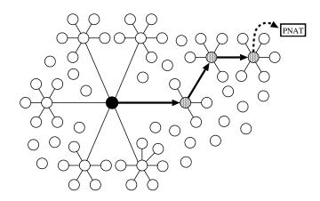
Figure 6: Mimic topology and traffic flows for k = 3: Each node has  $\kappa \approx 6$  mimics (shown connected by solid lines). A node establishes its tunnel over mimic links (arrows in bold) and completes it with a random PNAT (dotted line). Nodes inject cover traffic with data traffic to yield a uniform total traffic T that flows bidirectionally over the solid lines. All packets on these links are pair-wise encrypted and padded to the same size.
