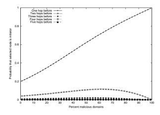
Figure 7: The malicious relay's confidence that a specific relay *i* hops before it is the tunnel's initiator, given  $\kappa = 6$  and tunnel length takes a Lognormal distribution with median 4,  $\sigma$  0.5.
